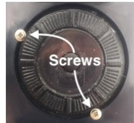
2. Remove the 2 screws that hold the Rotary Dial in place.
